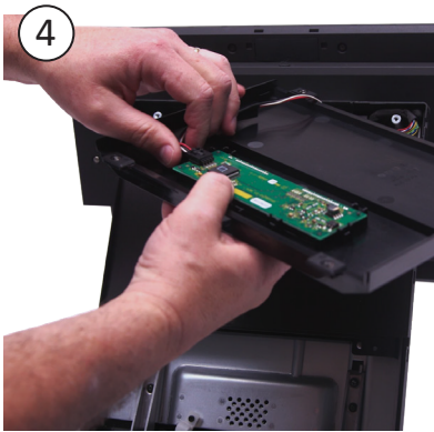
4 Remove the connector attached to the panel and tuck the wires into the exposed receptacle.
