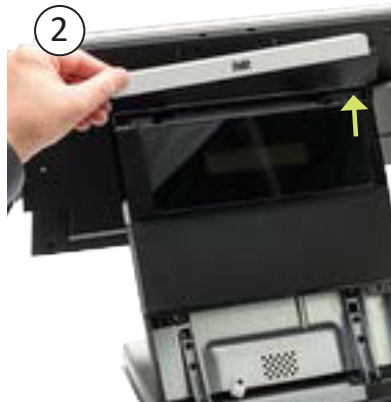
2 Remove the top strip by lifting it off of the terminal.
