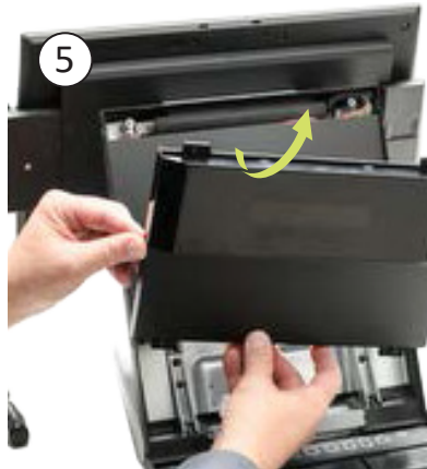
5 The panel can now be removed and set aside.
