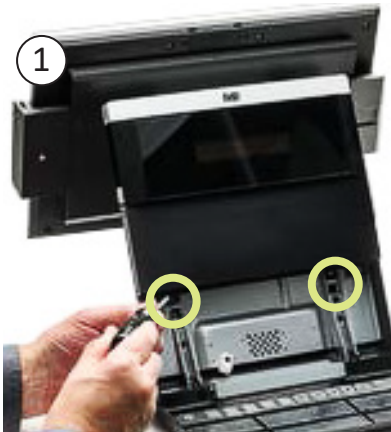
1 Remove the two screws as shown and set aside.
