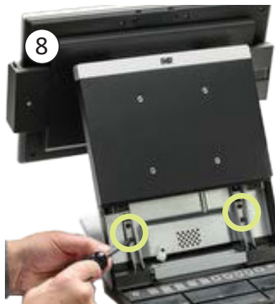
8 Remove the screws at the base of the mounting plate. Pull the display off of the pedestal to mount.
