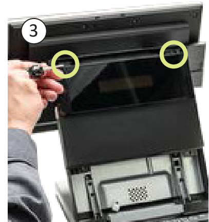
3 Remove the two screws as shown and set aside.
