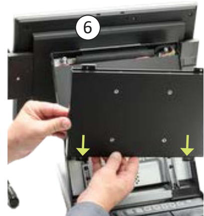
6 Insert the mounting plate base tabs into the drilled screw slots as shown.
