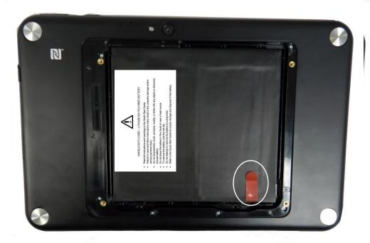
▲ DO NOT use any tools or sharp instruments to remove the battery door, as this will cause damage to the battery and/or cause serious personal injury.
