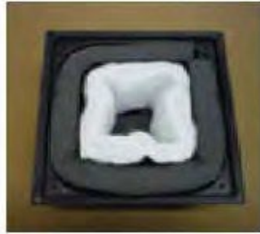
Fig.2 Install 3M foam and acoustic insulation.
