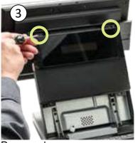
Remove the two screws as shown and set aside
