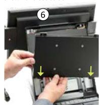
Insert the mounting plate base tabs into the drilled screw slots as shown
