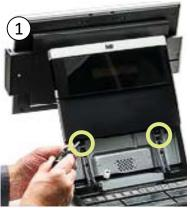
Remove the two screws as shown and set aside
