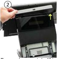
Remove the top strip by lifting it off of the terminal
