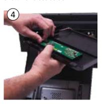
Remove connector attached to the panel and tuck the wires into the exposed receptacle
